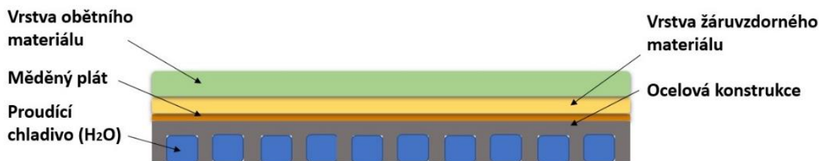
Obr. 23 – Element podlahy lapače koria ALLEGRO [30]
